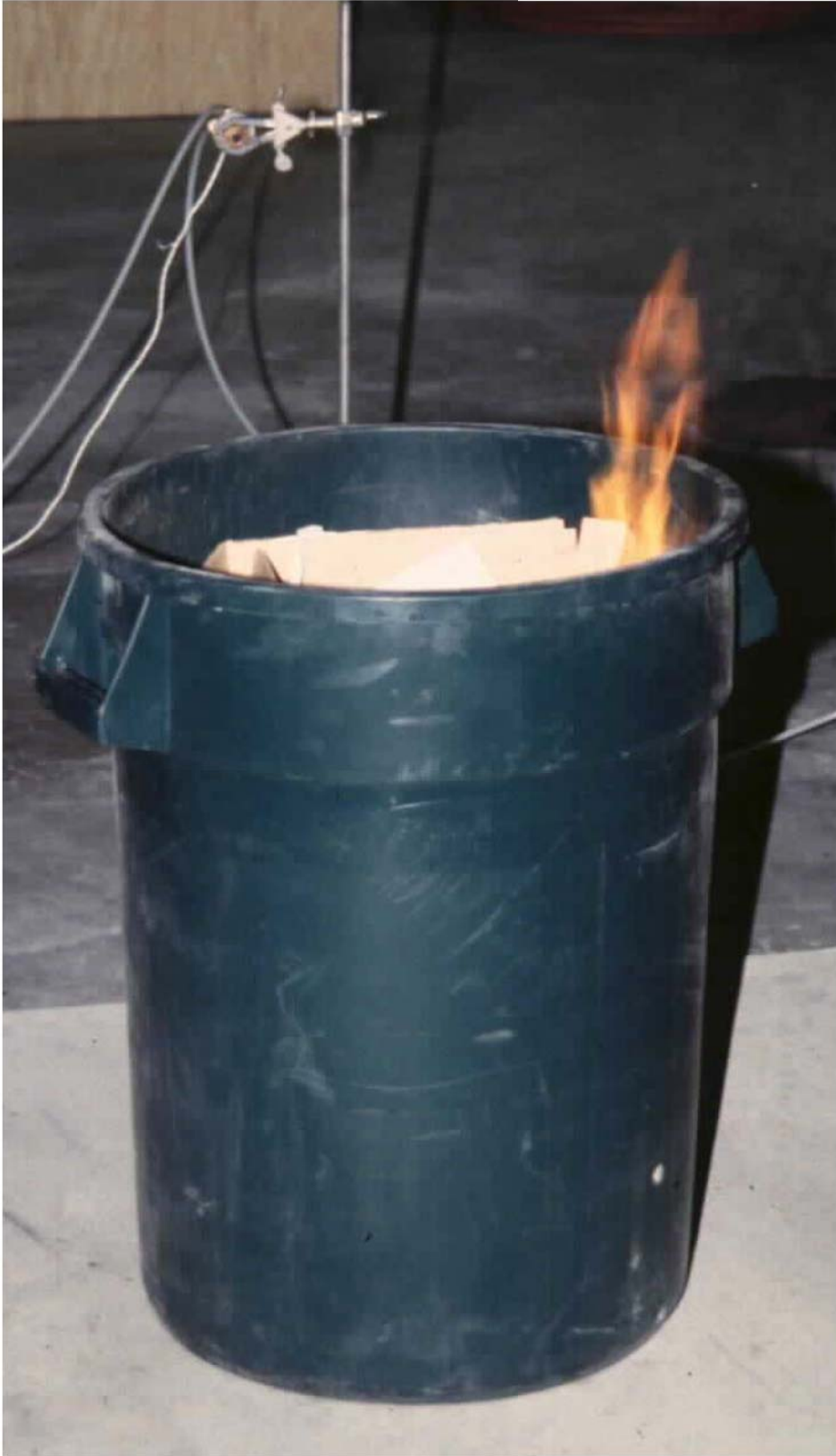
Figure 4. Fire developing in Trash Container 1.
