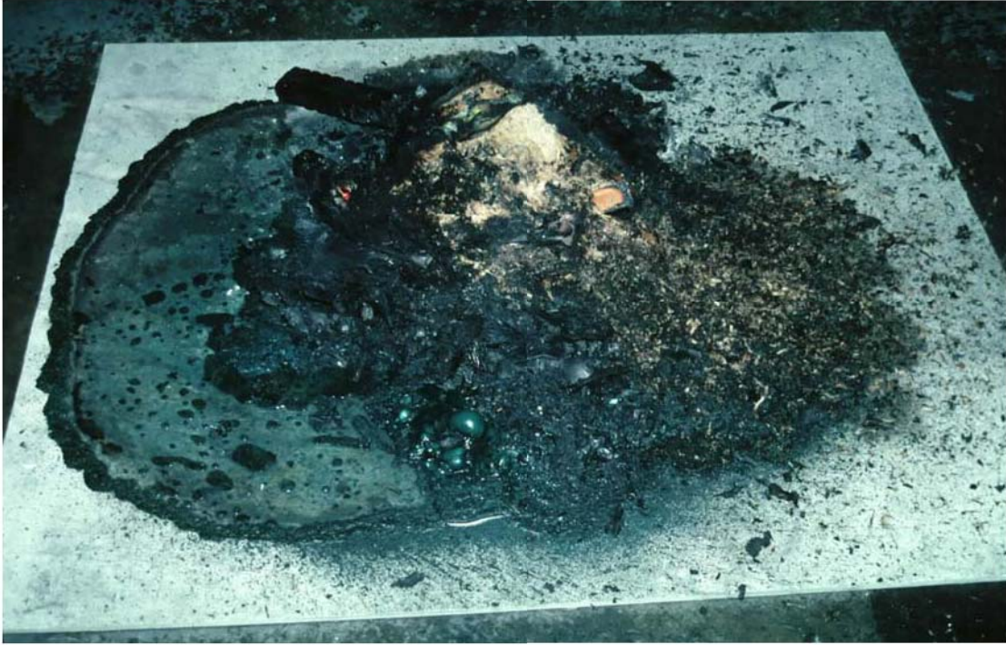
Figure 9. Remains of Trash Container 1 after test.
